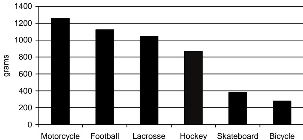
FIGURE 2—Typical weight comparison for several types of helmets as typically worn with face protectors, shields, etc.
