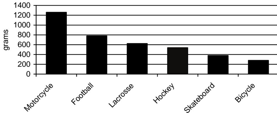
FIGURE 1—Typical weight comparison for several types of helmets.
