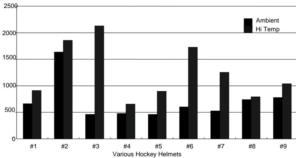
FIGURE 3—Comparison of hockey helmet performance at ambient and high temperature-side impacts.
